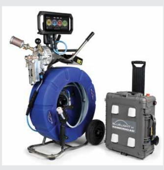
is a very focused range of visible light: **444 to 457 nanometers** (nm). This makes a huge difference in the quality and speed of the cure, and its why HammerHead's light-curing system uses Bluelight rather than UV.
