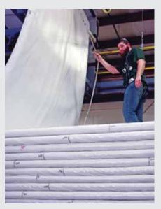
**DURAFLEX LINERS**–A wide range to accommodate varying bends, lengths and diameter changes. These single-layer felt liners with an array of polymer choices for your particular resin system, are best suited for on-site, vacuum impregnation in plumbing applications. These heat- or ambient-cured liners are highly flexible and available in custom lengths.
