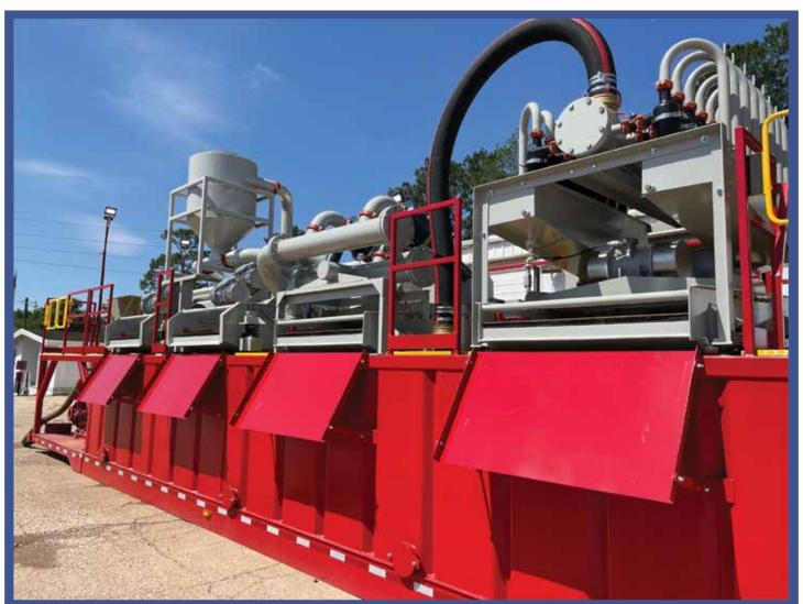
Triflo MFS8000: 3-phase drill mud cleaning and mixing machine with 8200 Gallon capacity, water flow-rate of 1000GPM and 750 GPM of drill mud
