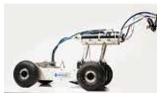
360Ringtech Robotics are capable of consistently applying high pressure, heated, fast set plural-component elastomeric polyureas and polyurethanes for use as liners in rehabilitation and new construction of liquid gathering, storage, and distribution systems. 360Ringtech provides true efficiency, reduced labor costs, and allows for the application of multiple products through a single device.
