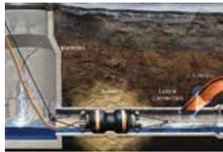
AV-100 Chemical Grout is an ultra-low viscosity, chemically reactive gel used to stop leaks, stabilize soil and control groundwater, by creating a long-lasting water barrier and superb soil stabilization. AV-100 has been successfully used for over 40 years to rehabilitate municipal sanitary sewer collection systems by eliminating infiltration in manholes, mainlines, laterals and lateral connections.
