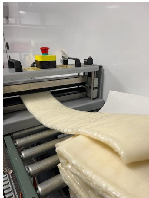
Calibrated, wet-out liner
