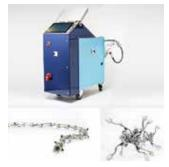
The KASRO UV CCU is a drum/control combination for 6" to 48" diameters. The KASRO UV light source chain 8 x 400W/600W and UV double cores 2 x 4 x 1000W can be operated to effectively cure GFP liners. The UV CCU is equipped with four wheels, making it mobile and compact, and easy to use even on difficult-to-reach construction sites. Operation, display and datalogging is possible via a 21" touchscreen PC.
