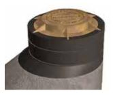
WrapidSeal™ manhole encapsulation system consists of an engineered primer and a unique, wrap-around, heatshrinkable sleeve designed specifically to seal joints and prevent groundwater from entering a collection system. WrapidSeal™ can be utilized on both new construction and rehabilitation of existing manholes.
